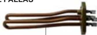
417449 (1 GR-230 VAC-2100W) 417137 (2 GR-230 VAC-3100W-SINGLE PHASE) 417450 (2 GR-230 VAC-3800W-THREE PHASE) 417438 (3 GR-230 VAC-4000W-SINGLE PHASE) 417451 (3 GR-230 VAC-5500W-THREE PHASE)
